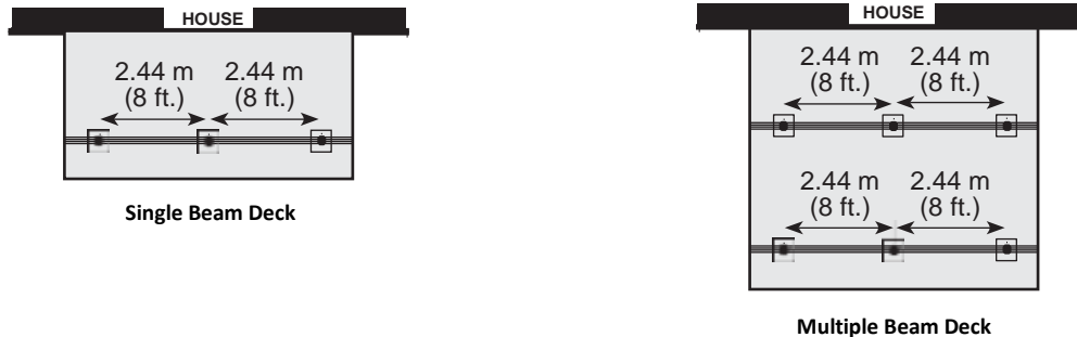
FIGURE 7 – Deck Beam Spacing
